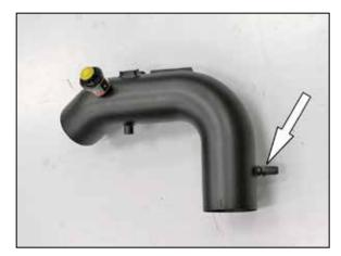
22. Install the 5/8 barb, 1/4npt crank case vent fitting provided into the K&N® intake tube as shown. NOTE: NPT fitting has tapered threads and only designed to be installed until hand tight, then tighten one rotation or when the fitting becomes difficult to return.
