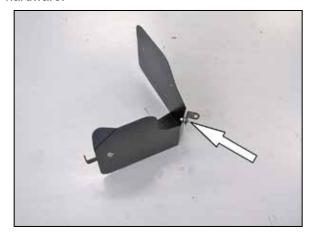
11. Install the tube mounting bracket (070712) onto the heat shield as shown using the provided hardware and spacer.
