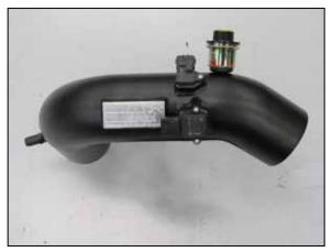
23. Install the inlet air temperature and mass air sensors into the K&N® intake tube using the provided hardware
