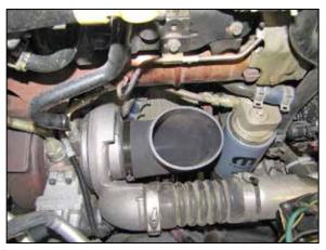
8. Install the K&N® elbow hose onto the turbo inlet and secure with the provided hose clamp.
