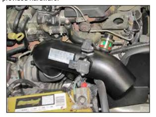
24. Install the K&N® intake tube assembly into the silicone hose at the turbo inlet and align with the mounting bracket installed on the heat shield. Secure the heat shield with the provided hardware and hose clamp
