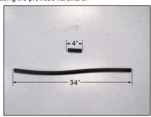
14. Cut the provided edge trim into two lengths. One length will be 34" long and one section will be 4" long.
