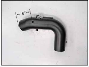
20. On vehicles equipped with a filter minder, drill a 5/8"id hole into the  $K\&N^{\odot}$  intake tube where shown.
