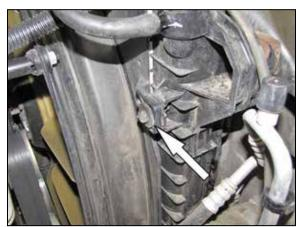
16. Remove the fan shroud bolt shown.
