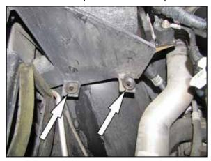
9. Remove the two air box mounting grommets shown.
