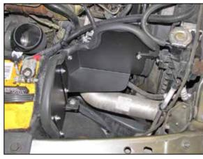
17. Set the heat shield onto the air box mounting tabs so that the inserts engage with the mounts, align the mounting bracket with the fan shroud mounting location and then secure the heat shield with the provided hardware.
