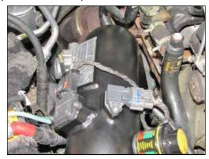
27. Reconnect the mass air sensor and inlet air temperature sensor electrical connections. NOTE: The factory wiring harness may need to be adjusted so that the harness is not too tight.
