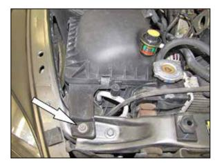
5. Loosen and remove the nut which secures the air box to the core support.
